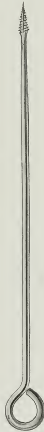
Fig. 29.—Long-Shank Screw-Porte. Without handle. The shank has a ring end for receiving a small bar as a handle.
